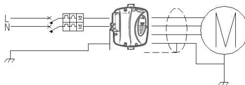
**EN** The device is provided with two terminals (line / pump) accessible through a door with built-in cable glands, which is connected to the device with screws. Remove the door, exposing the terminal and passing the cables in their cable glands:
